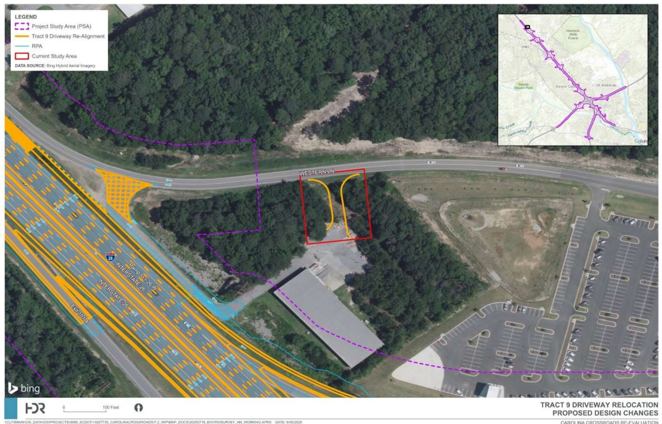
Figure 6. Tract 9 driveway realignment
