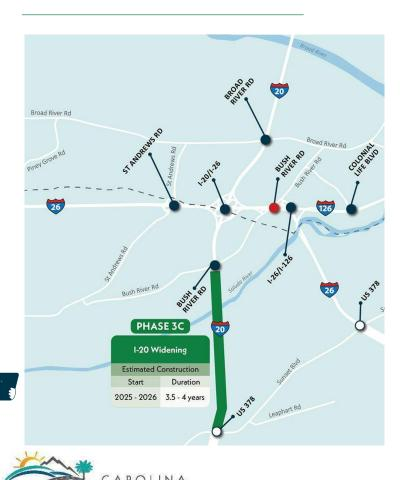
Phase 3C of the Carolina Crossroads Project is a design-build project. The scope of work focuses on the reconstruction of both the eastbound and westbound lanes of I-20 from US 378 to Bush River Road, primarily involving mainline interstate and ramp reconstruction and improvements, without significant interchange work.
