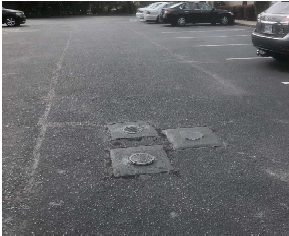
Photograph 11 – View of monitoring wells located in the parking lot of the Affordable Dentures and Implants business near the proposed new ROW area #5.
