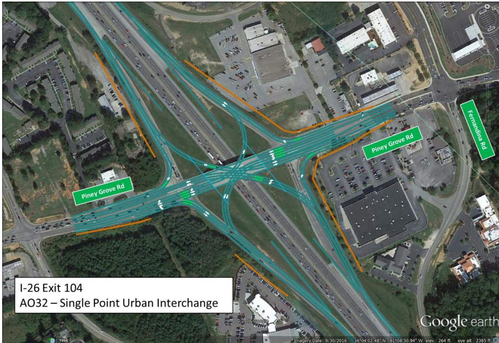
Figure 3-42 - AO32: Exit 104 Single Point Urban Interchange
