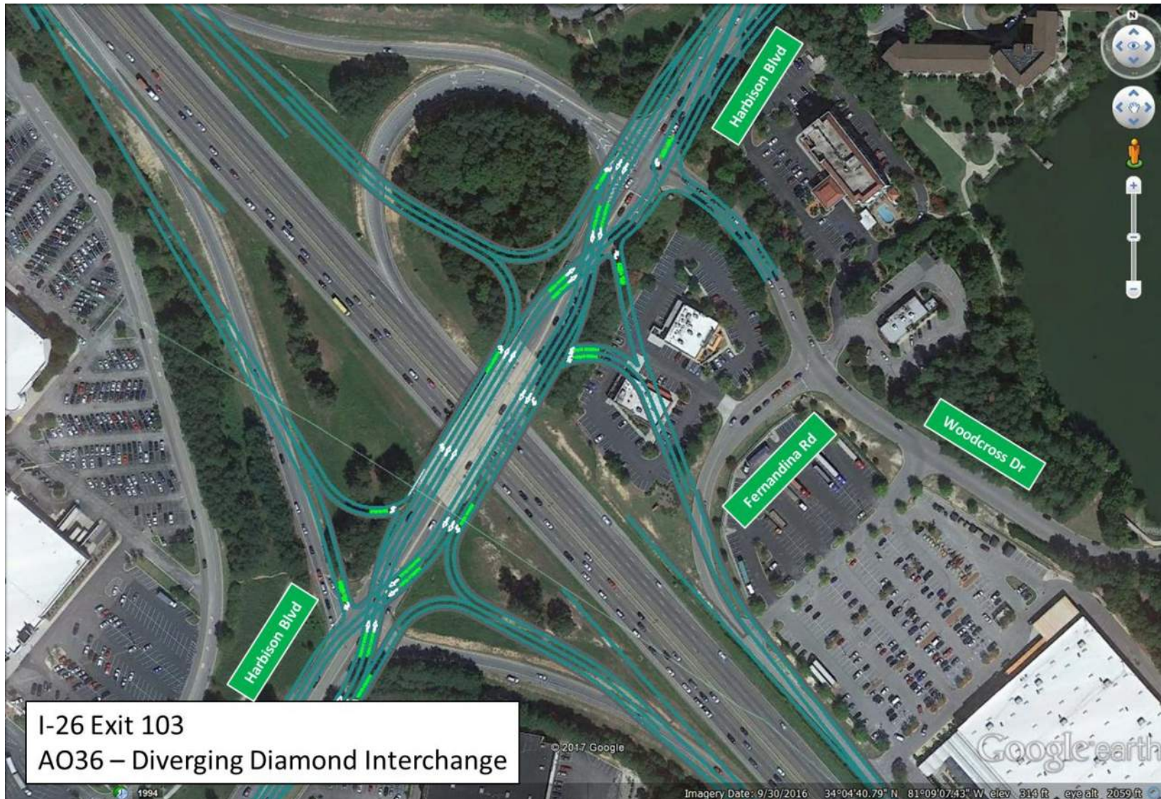
Figure 3-46 - AO36: Exit 103 Diverging Diamond Interchange
