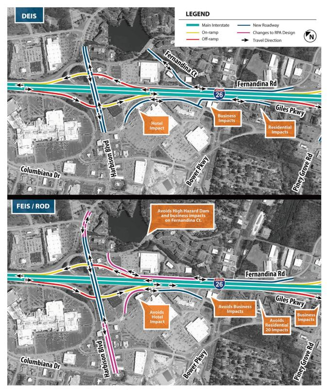
Figure 4-6A Design changes to RA1 – at I-26/Harbison Interchange
