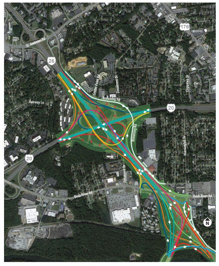
Figure 27: I-26 at I-20, Semi Directional 2 Loops
