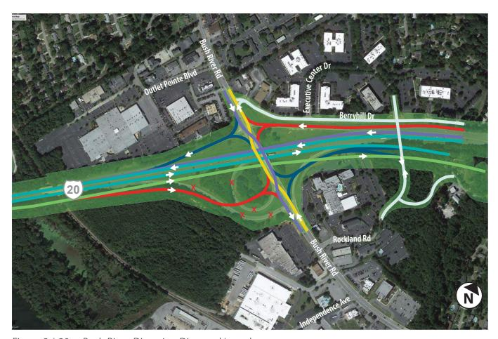
Figure 8: I-20 at Bush River, Diverging Diamond Interchange
