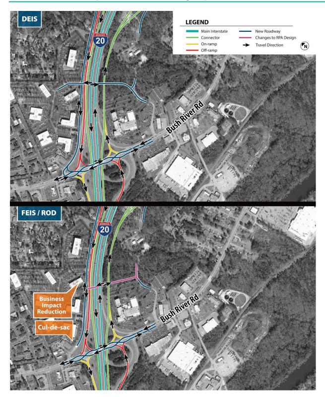
Figure 4-6E Design changes to RA1 – I-20/Bush River Road Interchange
