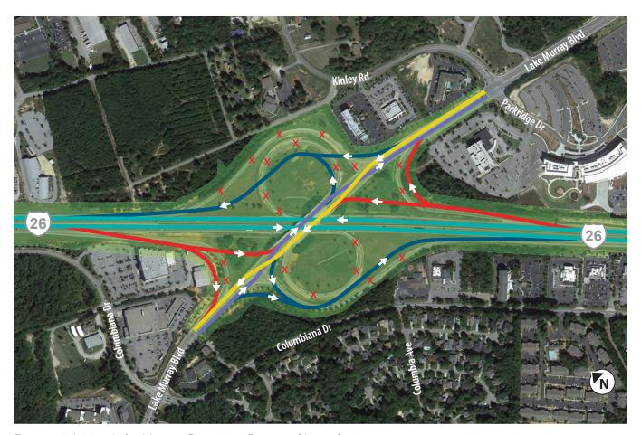
Figure 50: I-26 at Lake Murray, Diverging Diamond Interchange
