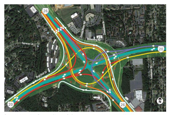
Figure 23: I-26 at I-20, Directional Interior Rights
