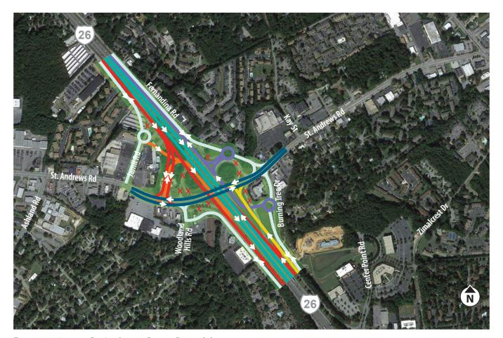
Figure 19: I-26 at St. Andrews, Ramp Roundabouts
