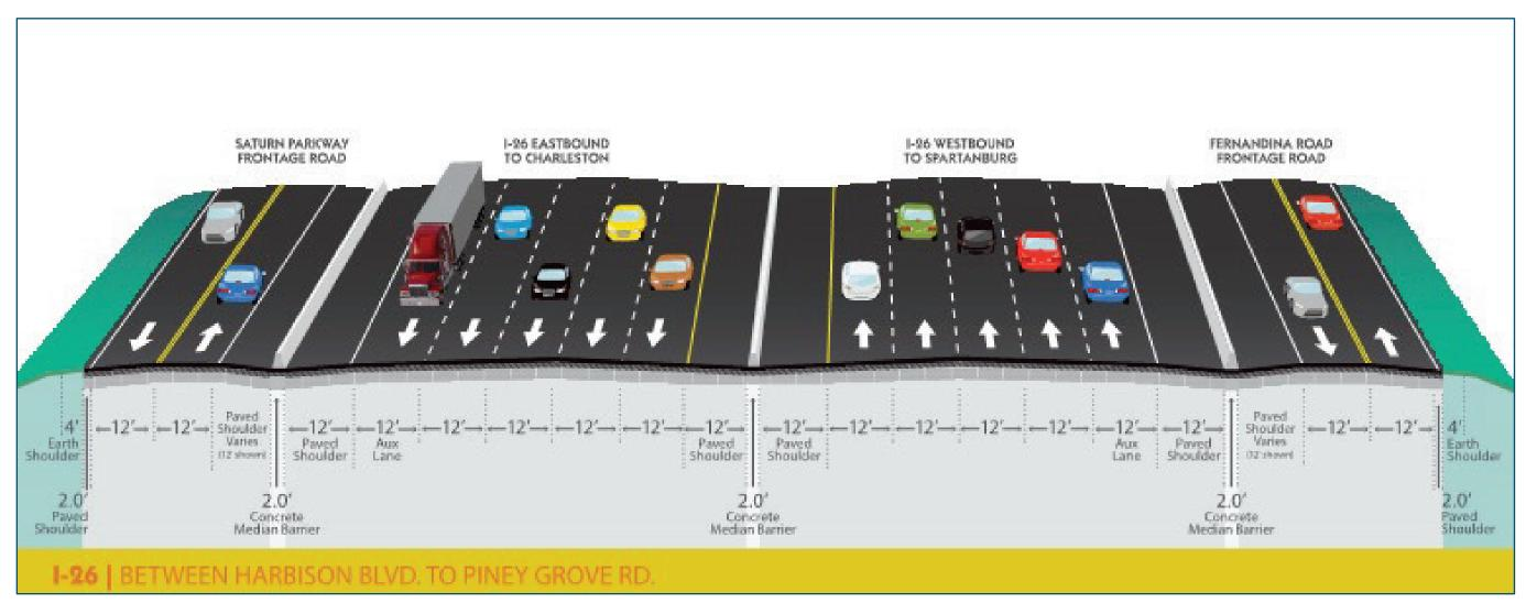
Figure 4.7 Proposed mainline alternative – collector-distributor lanes
