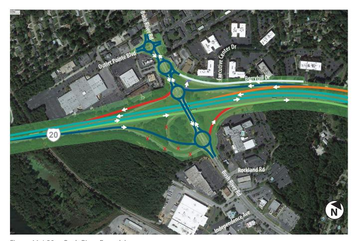
Figure 11: I-20 at Bush River, Roundabouts
