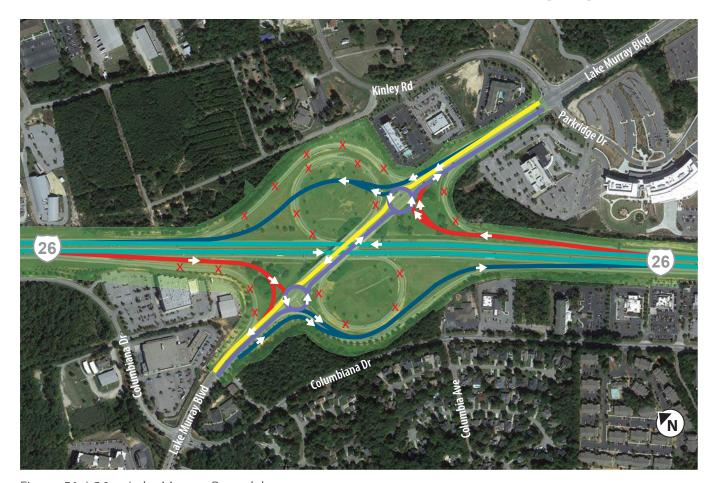
Figure 51: I-26 at Lake Murray, Roundabouts
