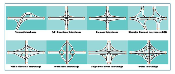
Figure 4.5 Preliminary interchange alternative designs
