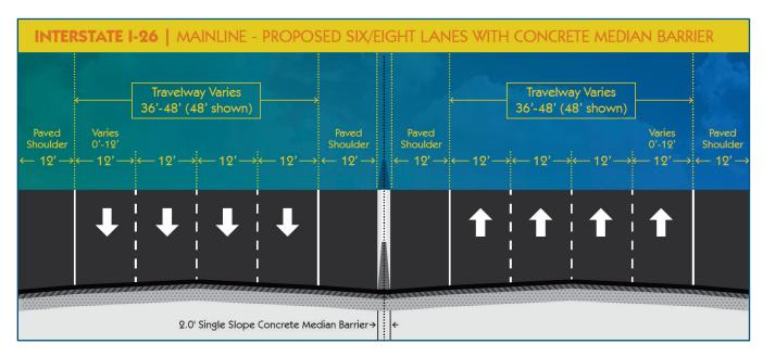
Figure 4.6 Proposed mainline alternative - six/eight-lanes with concrete median barrier
