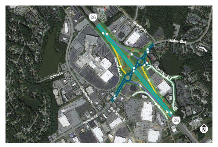
Figure 47: I-26 at Harbison Boulevard, Roundabouts
