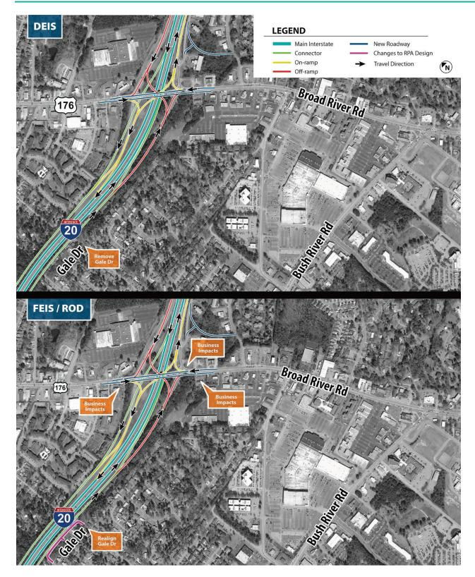
Figure 4-6D Design changes to RA1 - I-20/Broad River Road and Gale Drive Realignment
