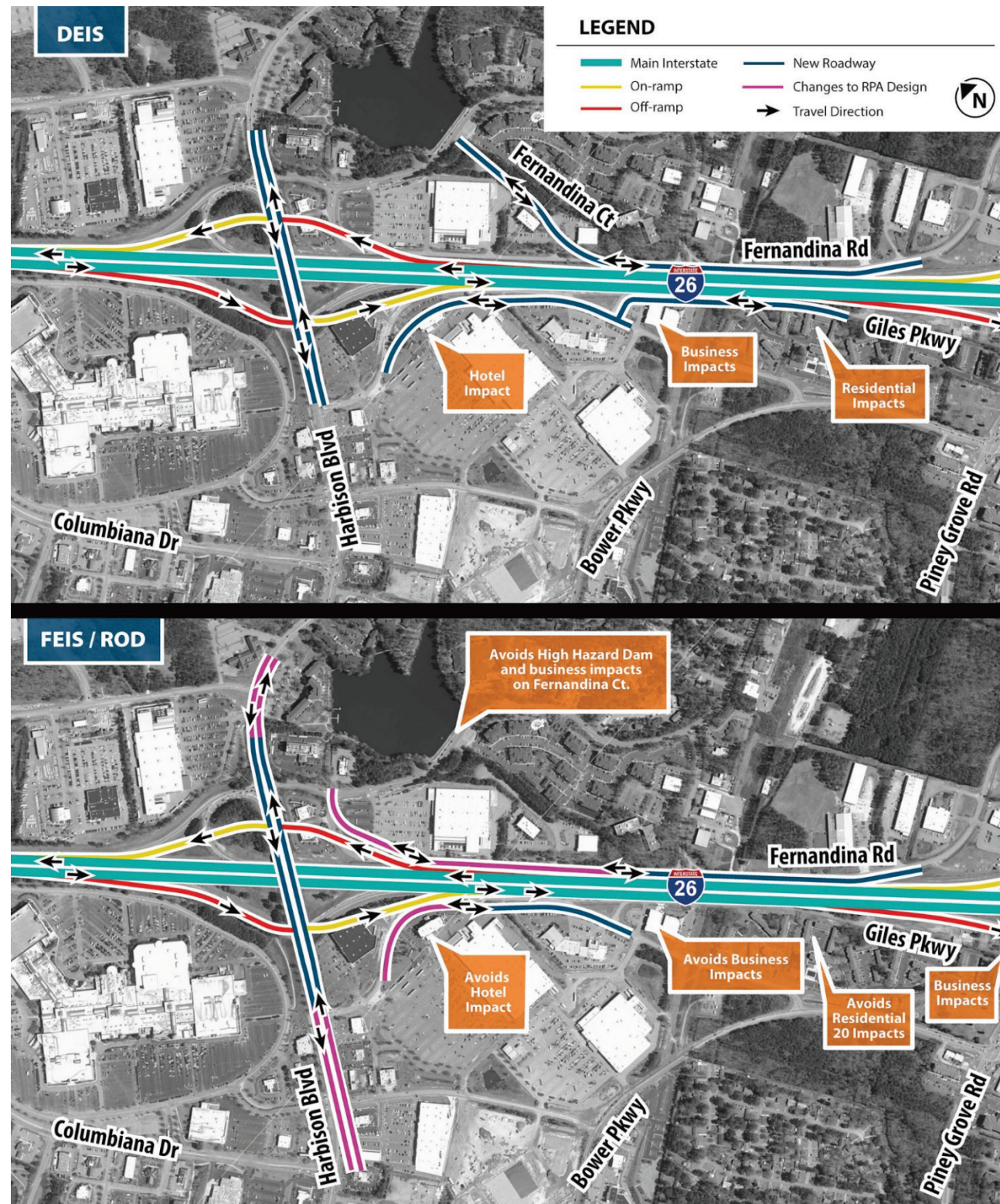
Figure 2-6A Design changes to RA1 – at I-26/Harbison Interchange
